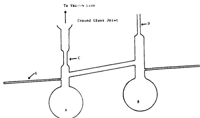
**Figure 4.** Apparatus used for the addition of salt to the anion radical solutions.
