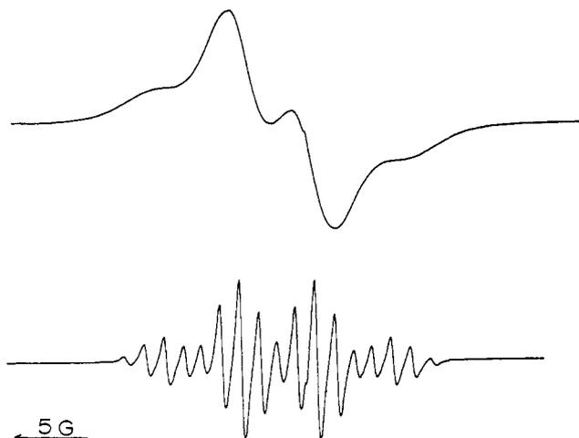
**Figure 3.** ESR spectrum of the TBCOT-HMPA-Na system. The lower spectrum was taken for the same anion radical solution but with added potassium iodide (0.2 M). Note the line narrowing upon addition of the potassium salt.
