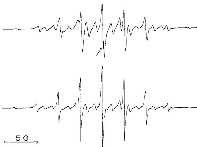
Figure 1. ESR spectra of the anion radicals formed by the reduction of a mixture of TBCOT and COT by sodium in HMPA. The lower was taken from the same anion radical solution but with added potassium iodide (0.1 M). Note that in the lower spectrum the concentration of COT<sup>•-</sup> is larger relative to that for TBCOT<sup>•-</sup>. The spectra were recorded at 25°. The spike indicated by the arrow marks 3391.2 G.
